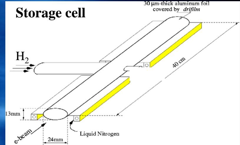
In previous experiments at VEPP-3 a polarized deuterium target was used. It consists of the ABS and storage cell was used to increase the target thickness.
