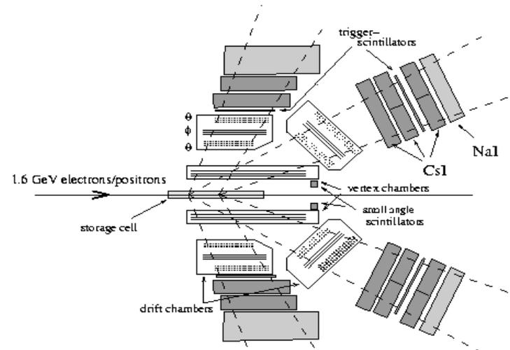
The detector for the measurement of  $(e^+p)$  and  $(ep)$  elastic scattering will be build on the basis of the detector used in the previous experiment. Scattered electron and recoil proton will be detected in coincidence, which allows to use kinematical correlations between their emission angles and energies. This is important for separation of the events from the process Under study from those of various background processes.
