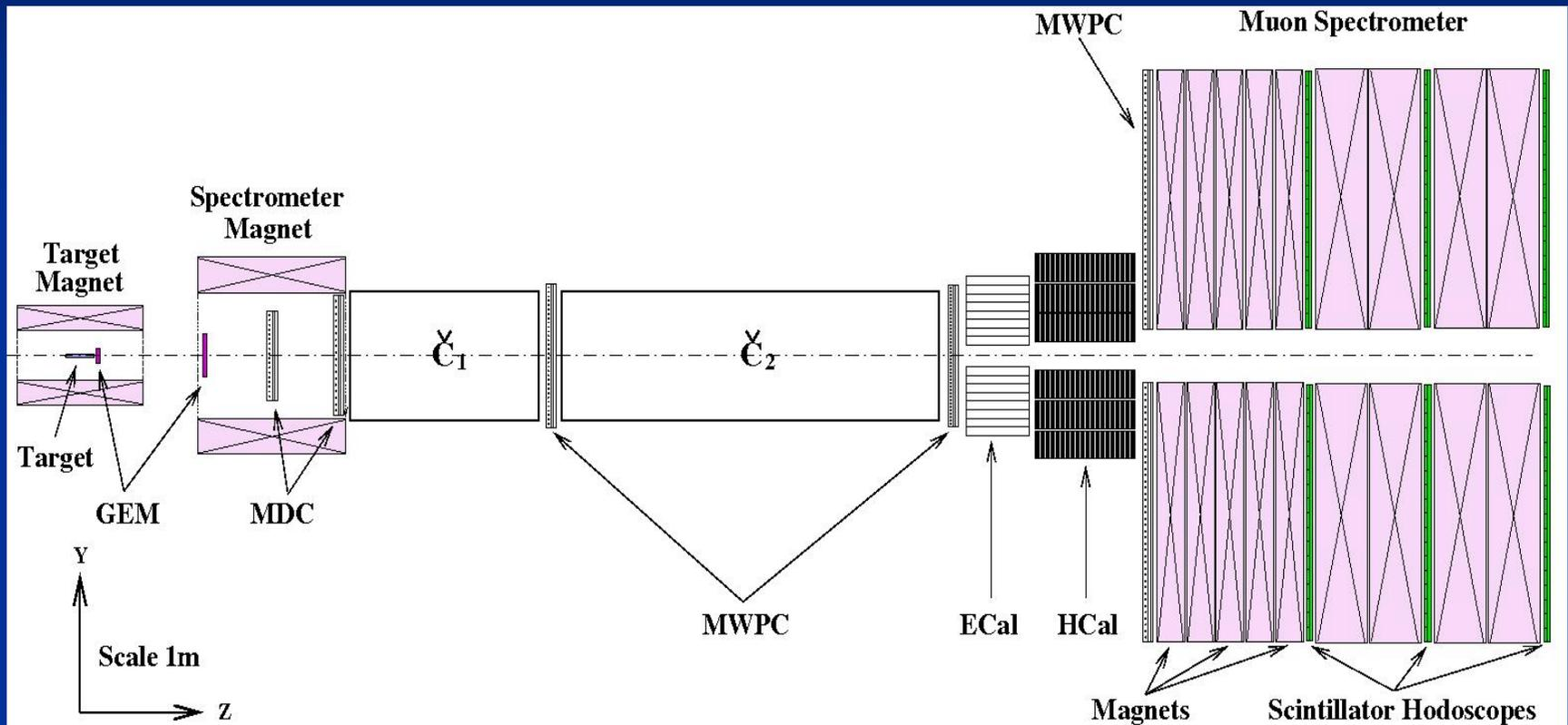
Two multi-channel threshold Cherenkov counters are added to distinguish between pions and kaons. However, acceptance is still significant for light resonances. Due to DAQ inclusive and exclusive reactions will be studied simultaneously.
