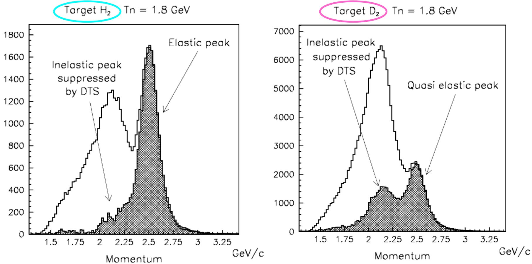
The rejection of the inelastic background using **DTS**. The **shaded hists** in the both figures present momenta spectra of charged secondaries when the signal from the DTS is in anticoincidence with the spectrometer trigger. The **transparent hists** show the same as ones but without the information from the DTS.
