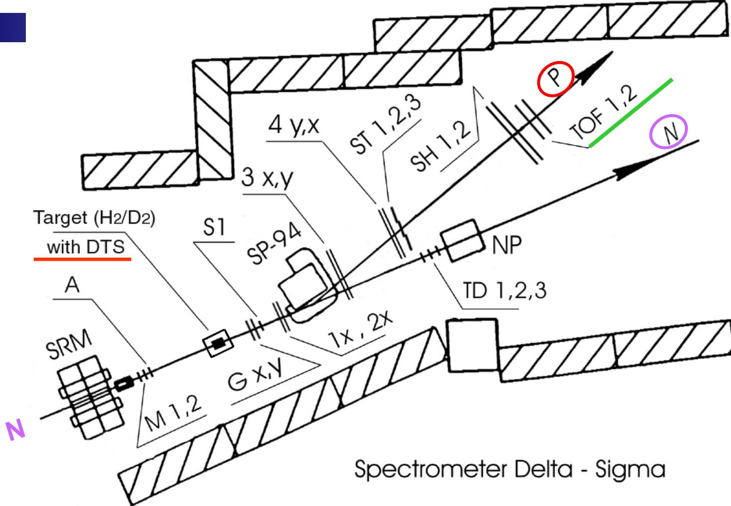
**Delta Sigma setup:** SP-94 - **analyzing magnetic dipole**; G<sub>x,y</sub>, 1x, 2x, 3x,y, 4x,y - **two sets of multiwire proportional chambers**; MPT-**polarized proton target** or liquid D<sub>2</sub>/H<sub>2</sub> target, surrounded by **DTS** system for detecting of  $\Delta$  recoils which decay to  $\pi$ , p and  $\gamma$ ; trigger counters – A, S1, ST1,2,3 and **time-of-flight system** – S1, TOF1,2, TD1,2,3 – **neutron transmission counters**, M1,2 – **monitors**.
