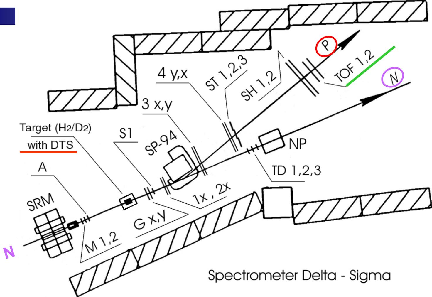
**Delta Sigma** setup: SP-94 - analyzing magnetic dipole; G<sub>x,y</sub>, 1<sub>x</sub>, 2<sub>x</sub>, 3<sub>x,y</sub>, 4<sub>x,y</sub> - two sets of multiwire proportional chambers; MPT-polarized proton target or liquid D<sub>2</sub>/H<sub>2</sub> target, surrounded by DTS system for detecting of  $\Delta$  recoils which decay to  $\pi$ ,  $p$  and  $\gamma$ ; trigger counters – A, S1, ST1,2,3 and time-of-flight system – S1, TOF1,2, TD1,2,3 – neutron transmission counters, M1,2 – monitors.
