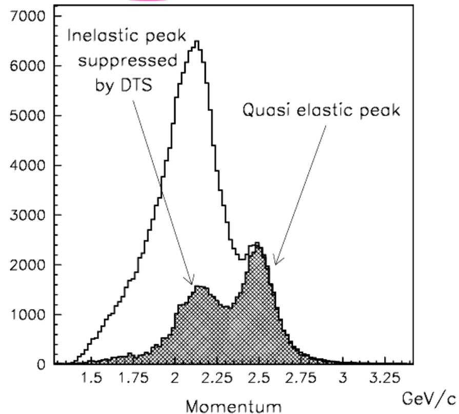
The rejection of the inelastic background using **DTS**. The *shaded hists* in the both figures present momenta spectra of charged secondaries when the signal from the DTS is in anticoincidence with the spectrometer trigger. The *transparent hists* show the same as ones but without the information from the DTS.
