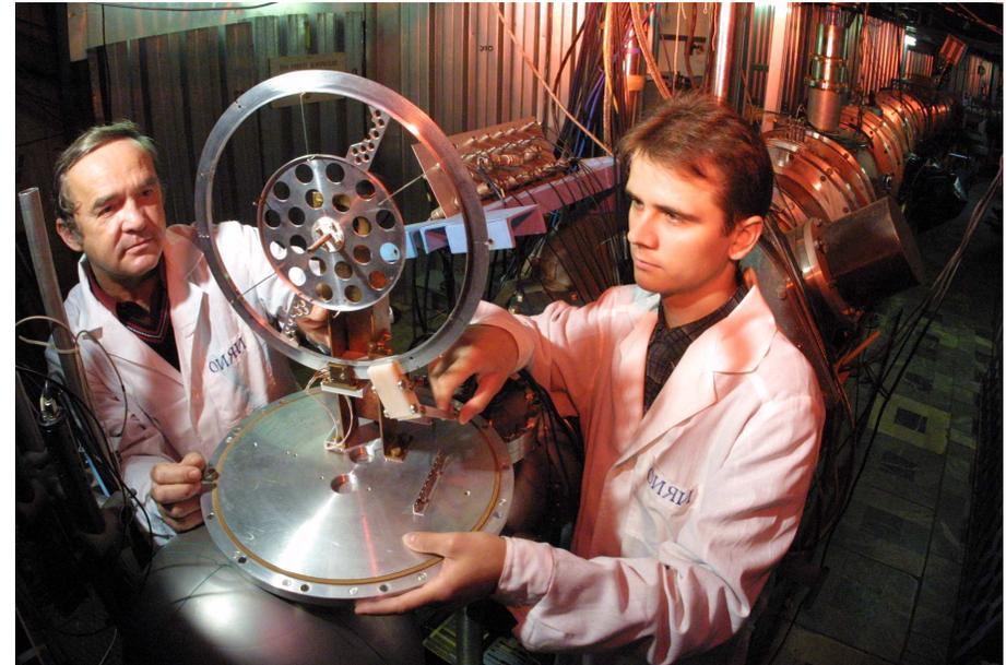
New Internal Target Station is very well suited for the measurements of the **dp**- elastic scattering observables at large angles in the cms.
