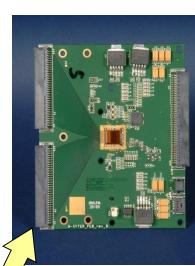
Front-end electronics board based on n-XYTER chip
