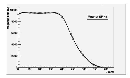
The field integral is 2 T·m at the max. current (1900 A) In March 2012 run the current up to 1570 A was used.
