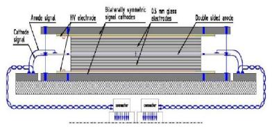
Symmetrical structure, differential readout
