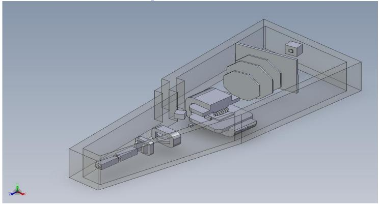
At the first stage of the experiment the existing magnetic optics: 2 lenses, 2 rotating magnets and large analyzing magnet of the 6V beamline will be used.
