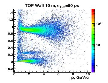
Au+Au @3.5 GeV Cu+Cu @ 5 GeV TOF baseline of 10m and resolution 80 ps provides the good PID Simulation- T.Vasiliev (LHEP-JINR) 15
