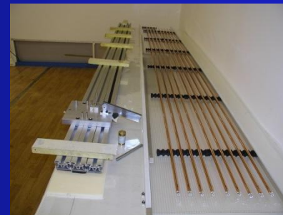
Straws under pressure test
