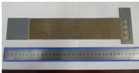
mock-up carbon-fiber ladder (15 g / 1m) and module circuit board
