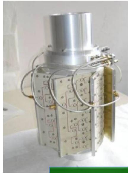
Slot-coupler RF structure (by IKP FZJ)
