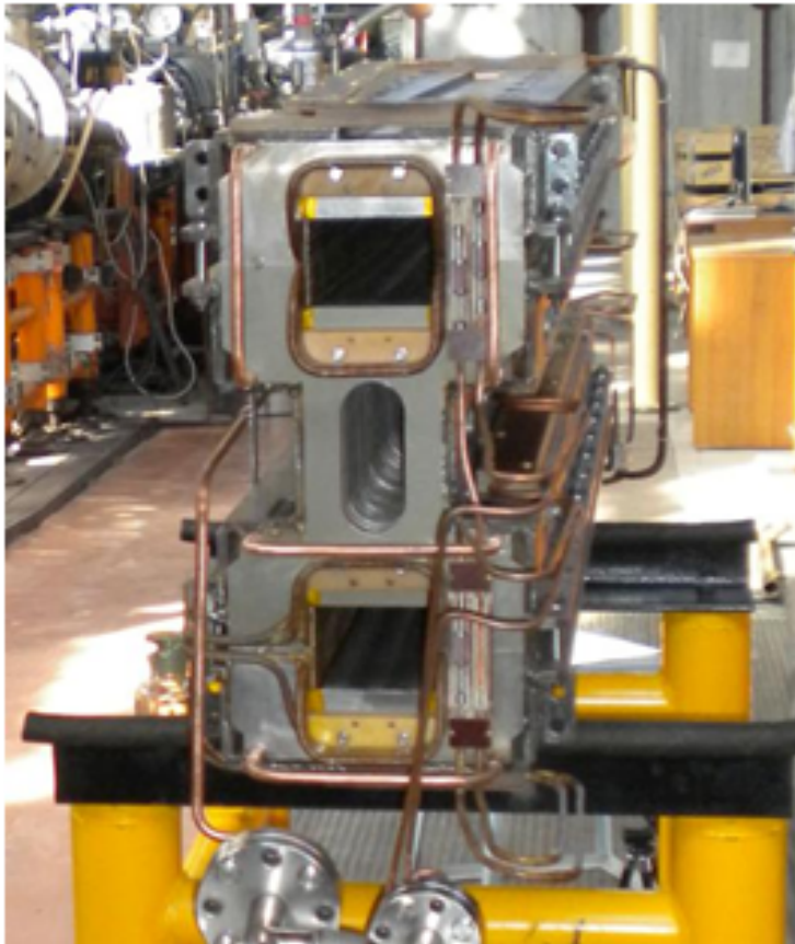
Test on vacuum tightness of the tubes for cooling the yoke
