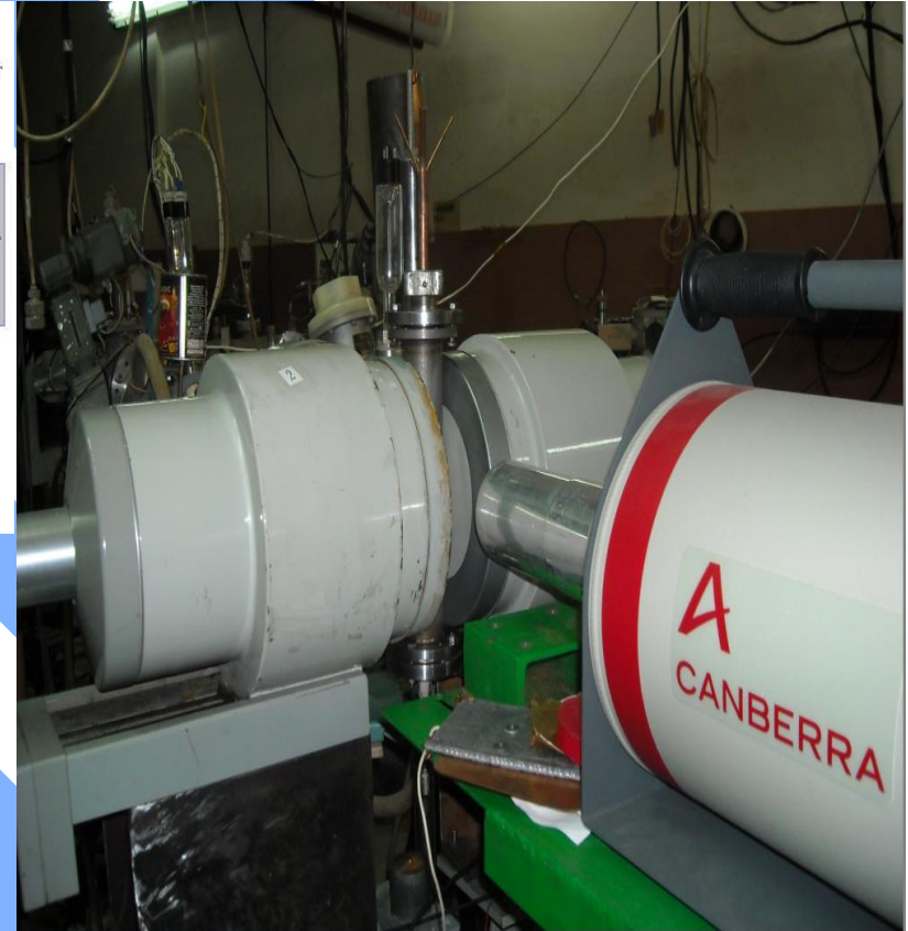
The multi-detectors set up, Vande –Graff accelerator.
