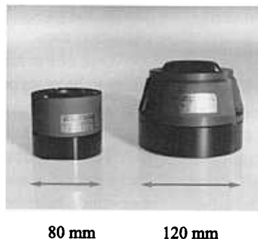
Fig. 2. Precise reference hole, specific sockets, quadrant-sensor target (type CERN) (CERN TS-SU-EM library and http://edms.cern.ch/nav/CERN-0000003489 )
