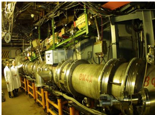
Fig. 5: Nuclotron (superconducting synchrotron)
