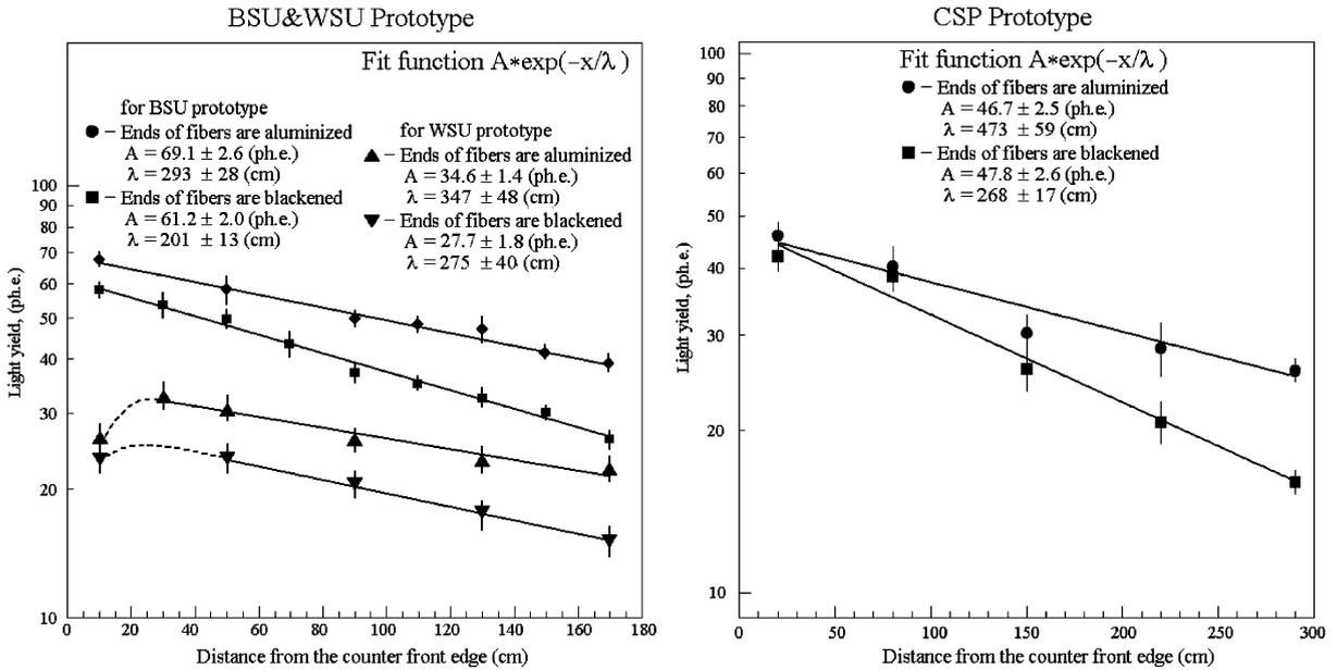
Fig. 5. Test results for the BSU ( $180 \times 17 \times 2 \text{ cm}^3$ ), WSU ( $180 \times 40 (30) \times 1.5 \text{ cm}^3$ ) and CSP ( $300 \times 30 \times 2 \text{ cm}^3$ ) counter prototypes. The light yield as a function of the distance to PMT.
