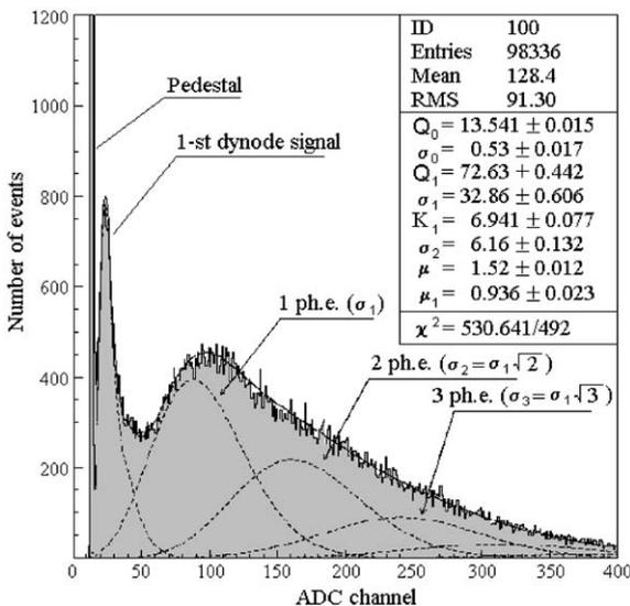
Fig. 14. A typical deconvoluted LED spectrum for the R5600 PMT.
