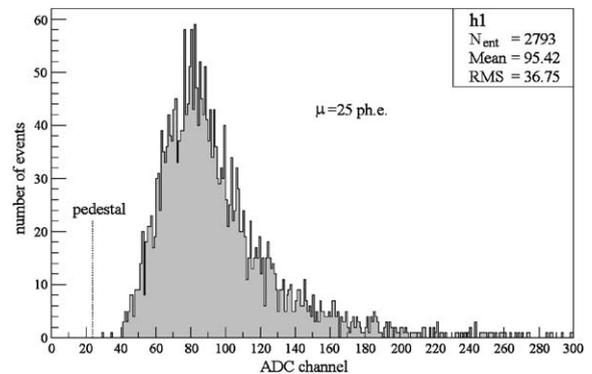
Fig. 15. A typical cosmic muons spectrum taken from the far end of a counter.
