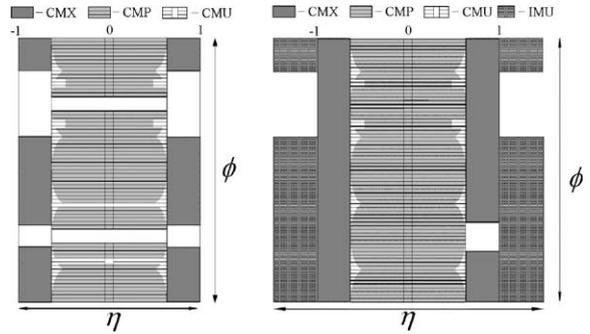
Fig. 3. Comparison of the muon counter coverage in Run 1 (left) and in Run 2 (right), as a function of the azimuth angle  $\phi$  and pseudorapidity  $\eta$ .
