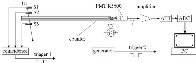
Fig. 13. Block diagram of the setup used for the counters test.
