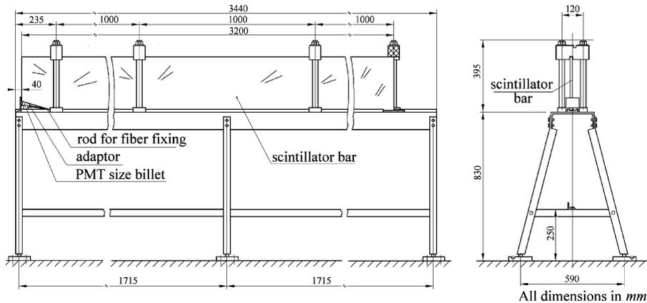
Fig. 11. Scheme of the assembly building-berth. Front and side view.
