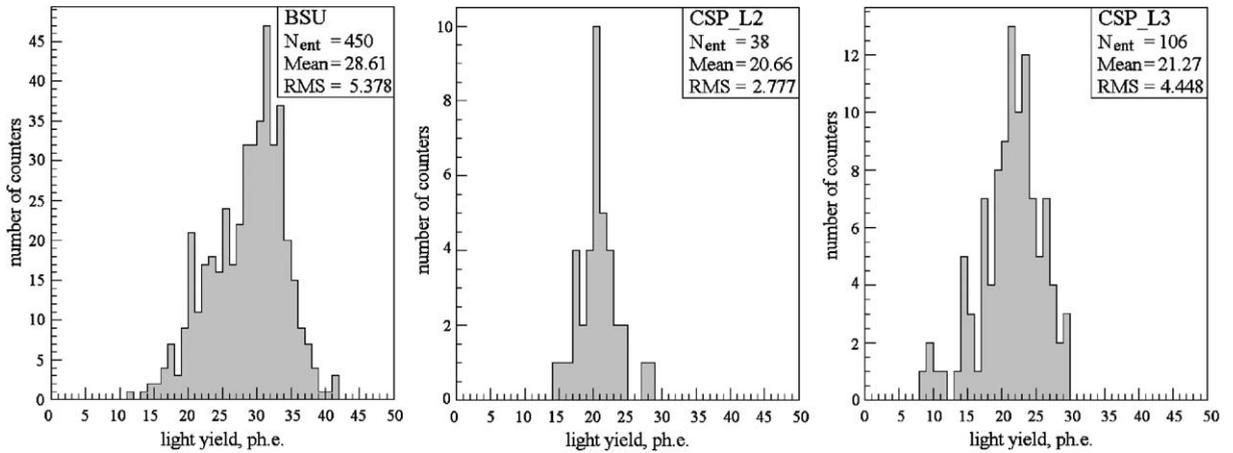
Fig. 16. Distributions of counter light yield from the far end for BSU, 310 cm long CSP L2 and 320 cm long CSP L3 counters, respectively.
