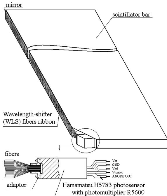
Fig. 4. Scheme of the counter layout employing a WLS fiber light guide.
