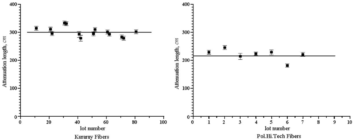
Fig. 10. The average attenuation length of Kuraray and Pol.Hi.Tech fibers as a function of the lot number.
