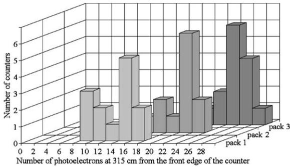
Fig. 6. Dependence of the light yield from the far end (in ph.e.) of CSP L3 counters from different Kharkiv scintillator lots. The scintillator bars quality improved by about a factor of 2 from lot #1 to 3. However, the light yield was in all cases good enough for our purposes.
