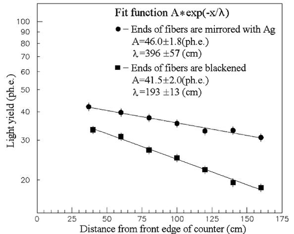
Fig. 7. Measurements of light yield of a BSU counter (15 WLS fibers, KURARAY type).
