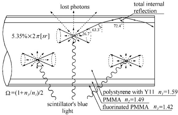
Fig. 8. Principle of the light collection employing WLS fibers.
