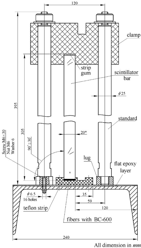
Fig. 12. Technical drawing of the clamping system.
