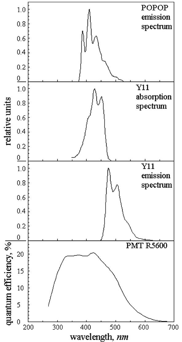
Fig. 9. POPOP emission spectrum, fluorescence converter Y11 (K27 formulation), absorption and emission spectra, and PMT R5600 quantum efficiency.
