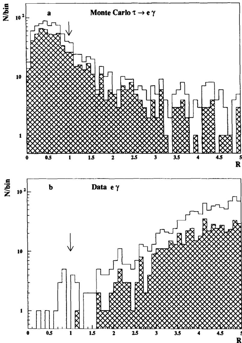
Fig. 2. Distribution in the variable  $R$  for  $\tau \rightarrow e\gamma$  candidates. a) Simulated events, b) data. Open histograms are before the background rejection described in Section 4.1, hatched histograms are after these requirements. No events remain in the signal region,  $R < 1$ .
