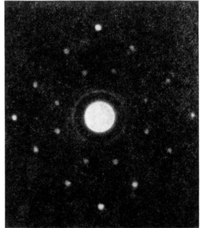
FIG. 1. Laue photograph showing neutron diffraction by NaCl.
