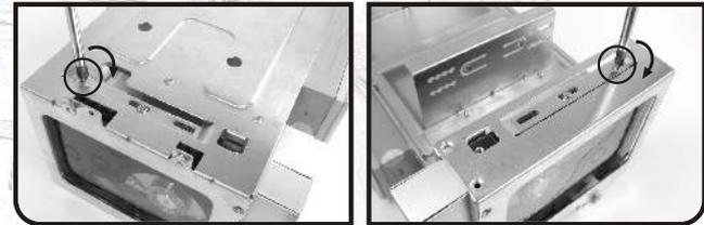
**3** A HDD can be installed on the side by securing 4 screws.
