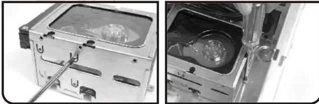
**4** Secure HDDs using screws when installing in the HDD rack.
