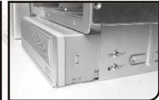
**3** When installing optical drives, it is recommended to screw into the 2nd hole as shown for a flush installation.
