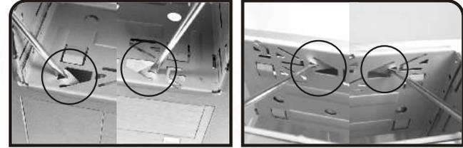
**4** Pull back all the metal clips for removing the cage.
