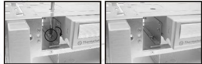
**8** Secure the top optical drive bay as shown.
