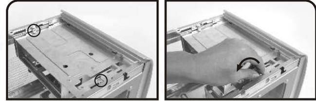
**1** Unscrew the 2 screws as shown to slide back the optical drive tray.
