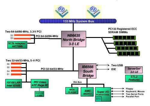
Figure 1-1. STL2 Server Board Block Diagram
