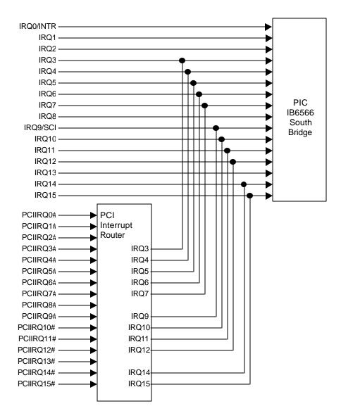
Figure 2-3. STL2 Baseboard Interrupt Routing Diagram (PIC mode)
