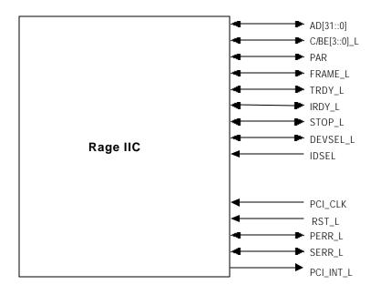
Figure 2-2. Video Controller PCI Signals
