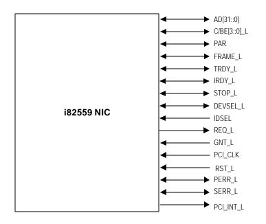
Figure 2-1. Embedded NIC PCI Signals
